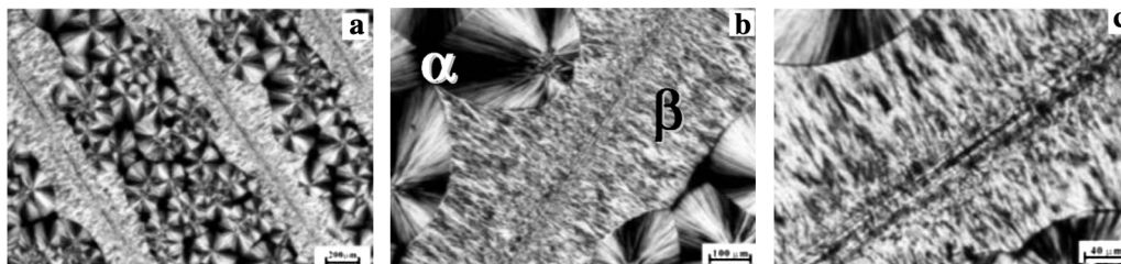
Fig. 20. Optical micrographs show the morphologies of an iPP fiber/matrix single polymer composite. The fiber introduction temperature was 173 °C. The crystallization temperature was 138 °C. Reproduced with permission from Ref. [195], copyright© 2003, American Chemical Society.
