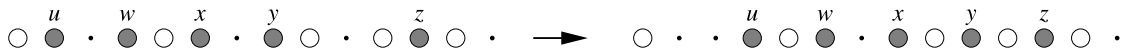
Fig. 5. The RightMove operation illustrated, applied to vertex u . The small dots indicate empty slots. Vertices are coloured according to the colour classes that they belong to.
