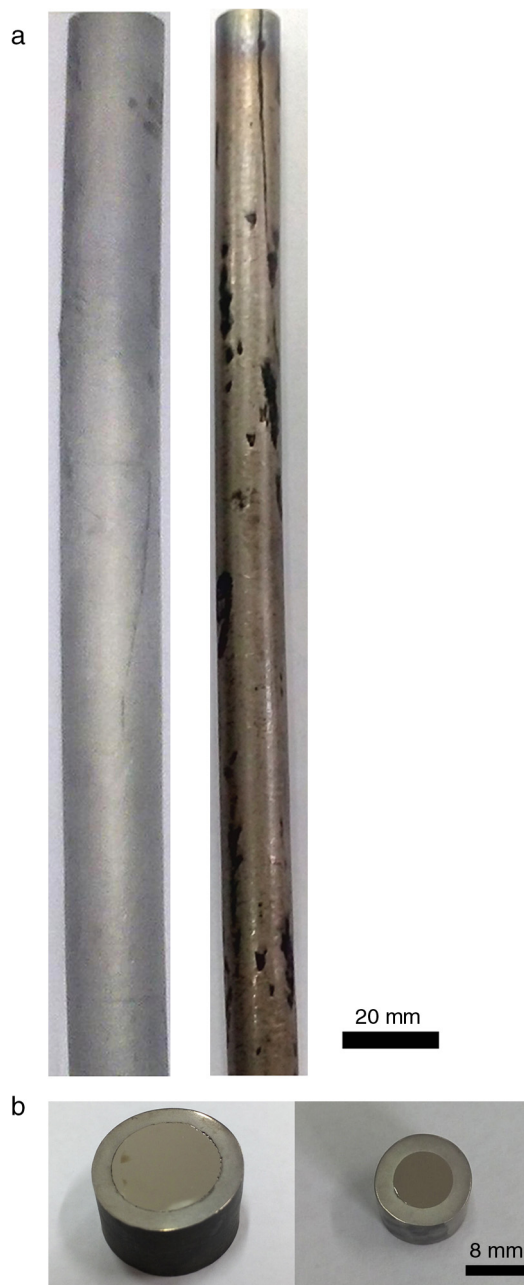
Fig. 1 – (a) Picture of the Ti/NiCr explosive cladding bars, (b) the corresponding cross-section images.
