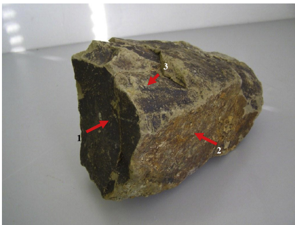
Fig. 12. Marl sample with three joint systems almost perpendicular to each other (first and third – secondary joints; second – bedding joints).
