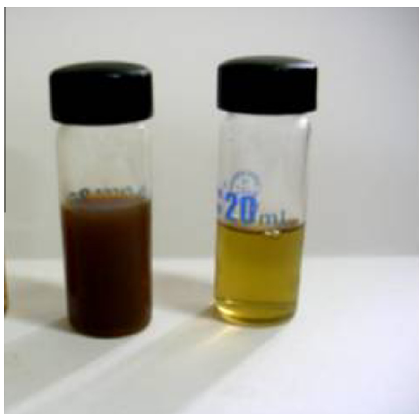
Figure 2 Color change of silver nitrate to silver nanoparticles (brown, left) by the addition of C. murale leaf extract (yellowish green, right).
