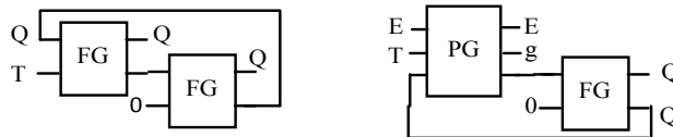
Fig.14.(a) Design of Reversible T-Latch; (b) Design of Clock enabled reversible T-Latch (T-FF)
