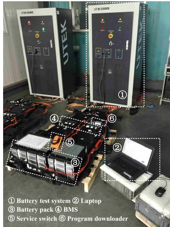
Figure 3 Laboratory battery test bench
