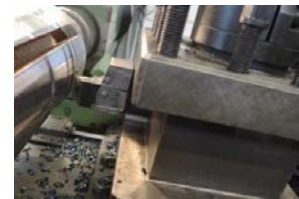
Fig. 3. Section of the work piece and the set-up utilized in the measurements.
