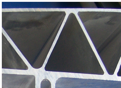
Fig. 1. Profile of extruded Al-0.6Mg-0.6Si aluminium alloy.
