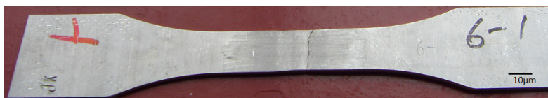
Fig.4. Tensile fracture sample of extruded Al-0.6Mg-0.6Si aluminum alloy, The thickness of the sample is 4mm.
