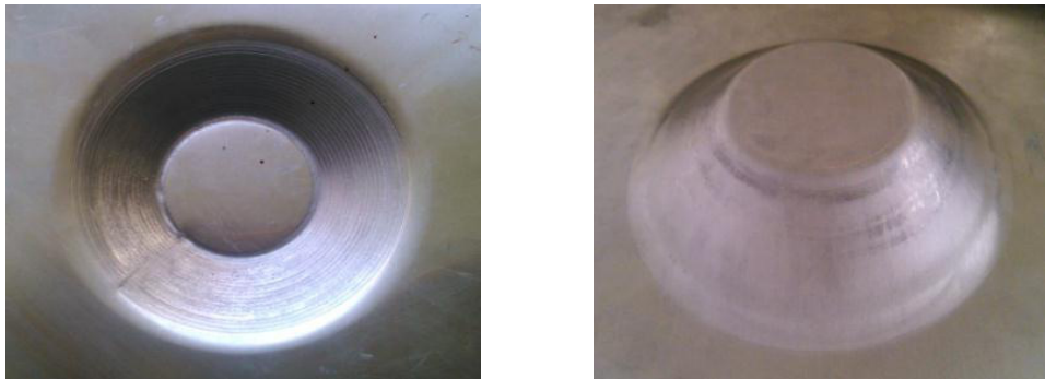
Fig. 3 Cone formed by increment forming process
