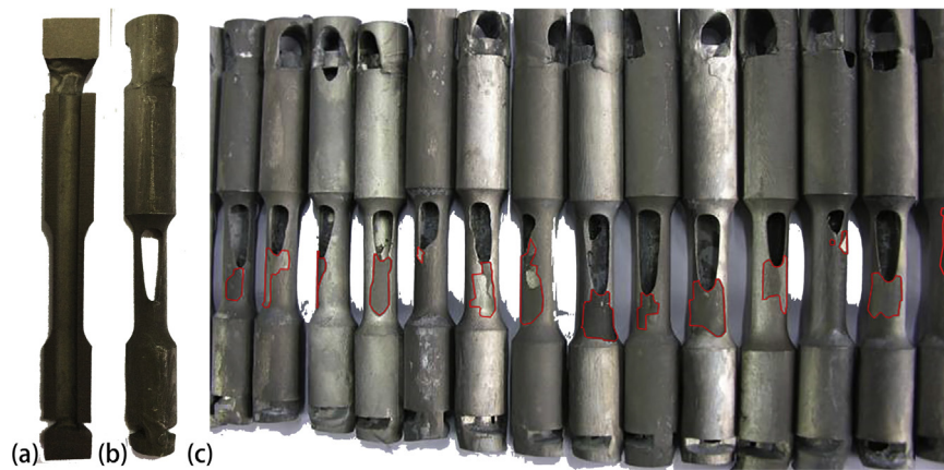
Fig. 21. Test bars with buckled cores: (a) core does not penetrate the wall; (b) core penetrates the wall; (c) RX grains (marked with closed red lines) in test pieces with penetrating core. (For interpretation of the references to color in this figure caption, the reader is referred to the web version of this article.)
