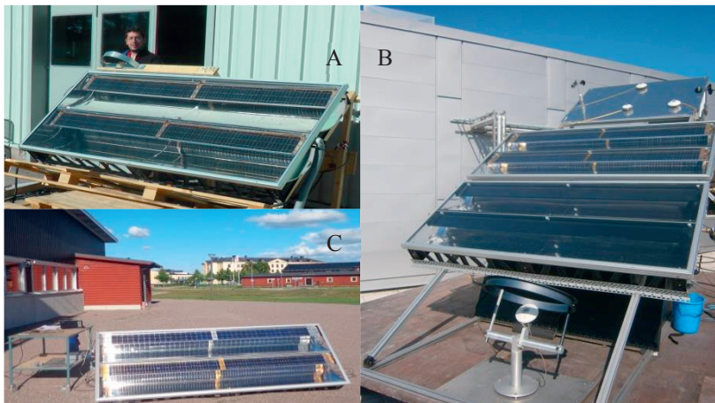
Figure 4. The outdoor measuring: (a) Solarus Factory PVT V1; (b) Darlana University PVT V2; (c) Gävle University PVT V3
