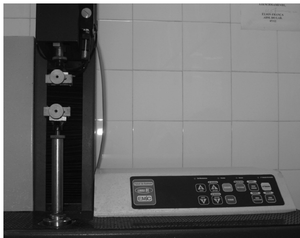
Fig. 3 – Axial traction test apparatus with 50 N load cell.
