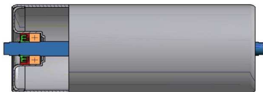
Fig. 1. Smooth idler for a belt conveyor with a labyrinth seal
