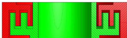
Fig. 2. Typical design of a labyrinth seal
