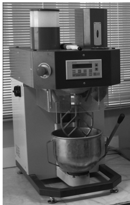
Fig. 1 Mechanical mixer used for preparation of specimens.
