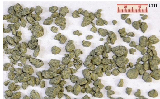
Fig. 1. The form of granular BRA modifier binder (pellets).
