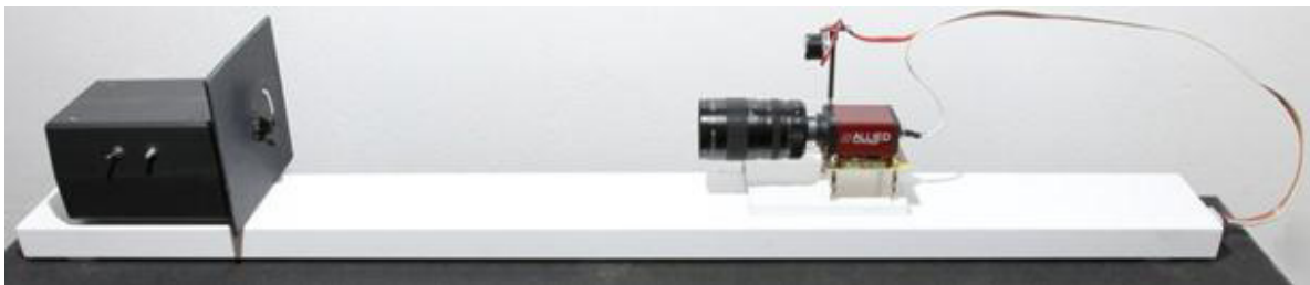
Fig. 6. Inspection camera AVT Marlin F-046B and measurement stand
