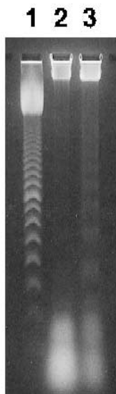
Fig. 6. Detection of DNA fragmentation in deferoxamine-treated F9 cells. Aliquots of 70 \mu\text{g} of DNA from deferoxamine ( 100 \mu\text{g/ml} )-treated (lane 3) and non-treated (lane 2) cells were electrophoresed in 2% agarose gels, and stained with ethidium bromide. Lane 1 is 100 bp ladder marker.
