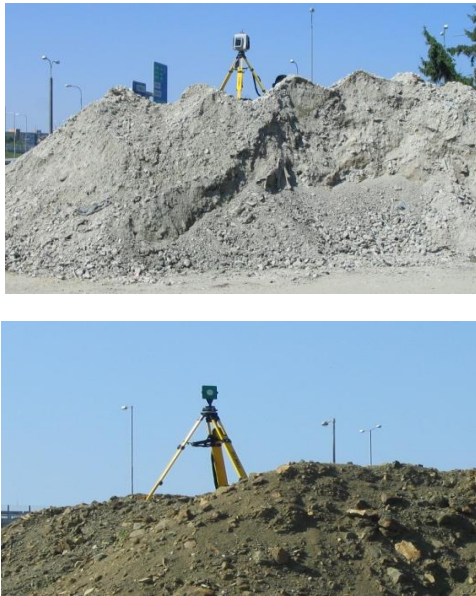
Fig. 4. The Trimble GX scanner (left) and the Trimble planar target (right)
