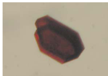
FIGURE 2 Photography of a crystal that looks like two agglutinated hexagonal plates. The crystal size along hexagon is 150 \mu\text{m} and thickness \sim 45 \mu\text{m} .
