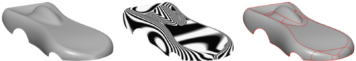
Fig. 17. Car model (GrabCAD, 2015). From left to right: The input model shaded and with reflection lines. The B-rep model consists of 42 NURBS patches, 14 of which have trimming curves that do not follow isoparameter lines. B-rep edges are shown in red. The model is topologically closed (it has no boundary), but it is not geometrically watertight. (For interpretation of the references to color in this figure legend, the reader is referred to the web version of this article.)
