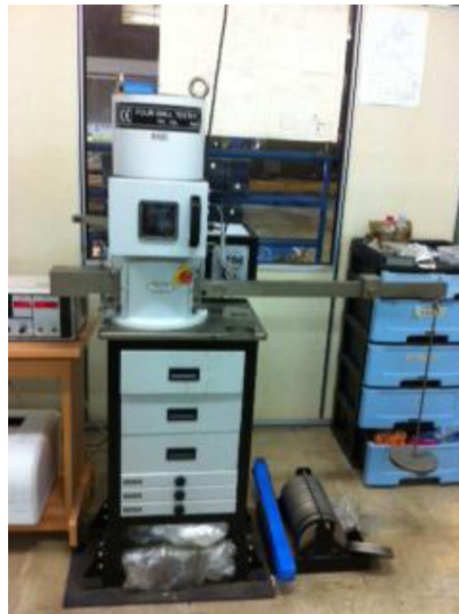
Figure 1: Four-ball tribotester machine.
