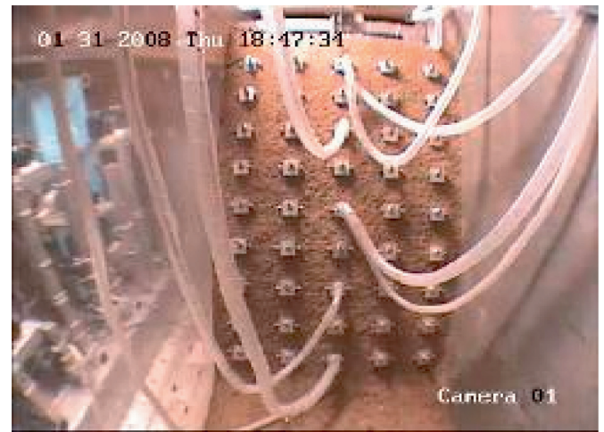
(b) Front view of the slope model in centrifuge test.
