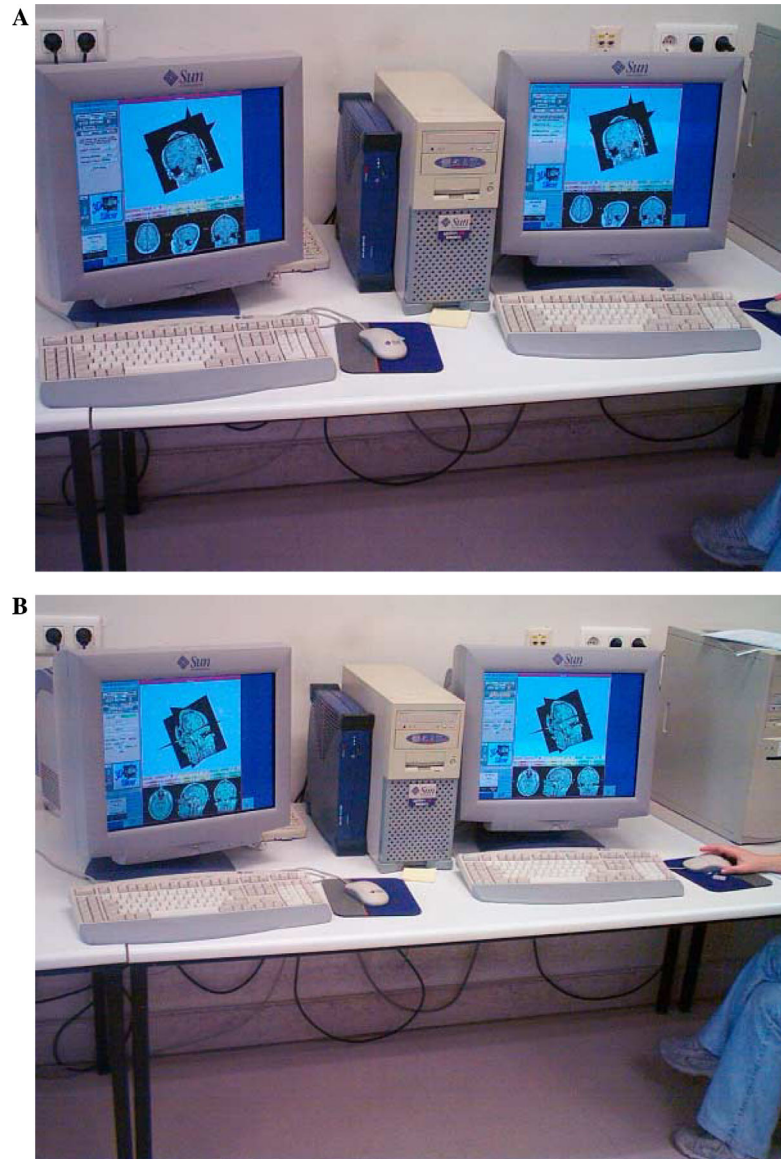
Fig. 7. (A) A mouse click on the computer on the right. The user starts dragging a slider to move the cutting plane. (B) Effect of the drag action: displays always remain coherent and the transition between both instants is smooth on both computers.
