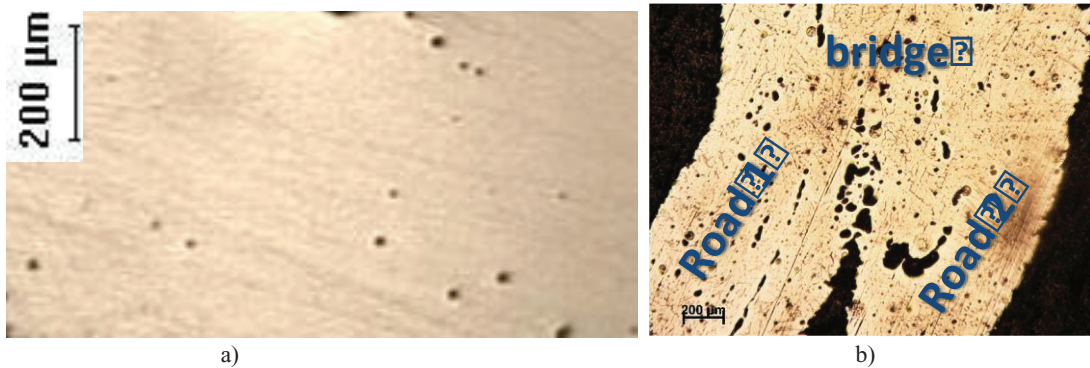
Figure 7: Detail of a micrograph of a sintered AISI 630 wire. a) Extrusion: pressure 20 MPa with 0.6 mm nozzle “C” at 180°C; Debinding: 10 h at 60 °C in water with anti-oxidation agents; Sintering: 15 hours at 1360 °C in hydrogen atmosphere; Result: 1 % porosity. b) Extrusion: pressure 11 MPa with 0.9 mm nozzle “B” at 180 °C; Debinding: 10 h at 60 °C in water with anti-oxidation agents; Sintering: 16 hours at 1360 °C in argon flow; Result: adhesion between roads, 10 % porosity, hardness 330 HV
