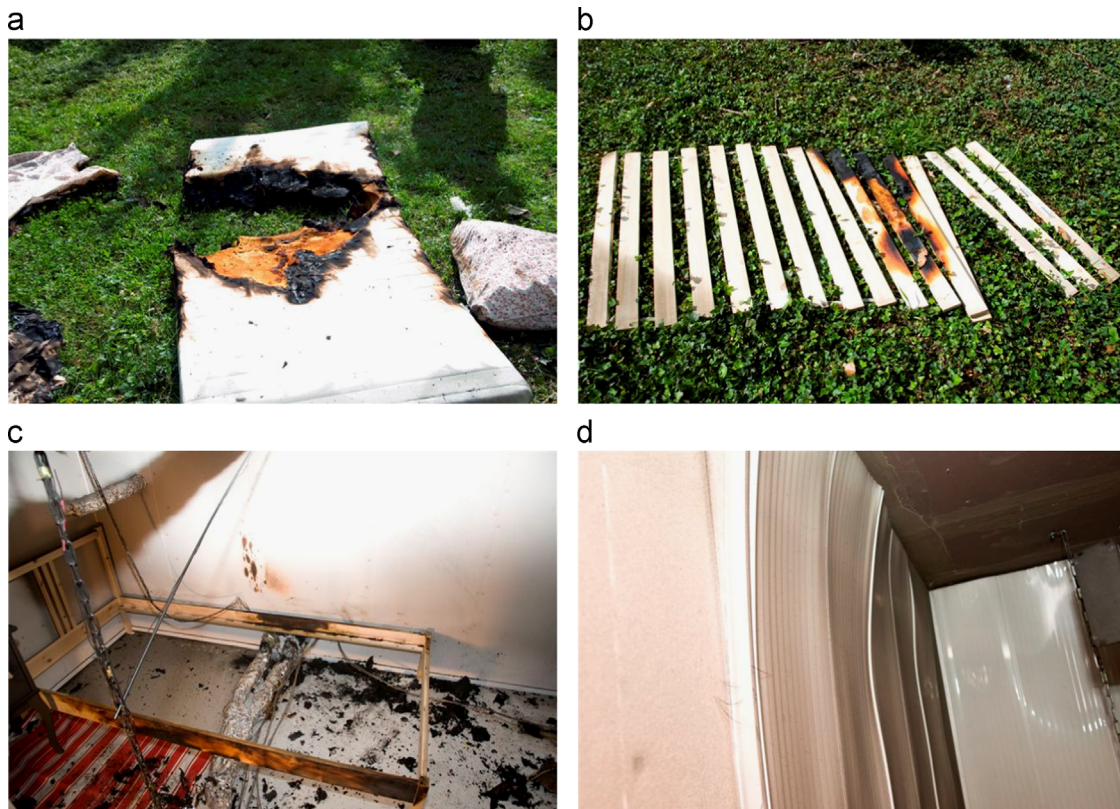
Fig. 7. Observations after test 1C: (a) mattress after test, (b) slatted bed base after test, (c) bed frame after test, and (d) deformation of PVC wall paneling.
