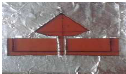
Fig. 4. Mask for Thin film coating using Aluminium foil.
