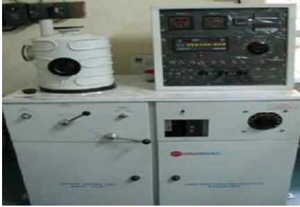
Fig. 5. Vacuum coating unit.
