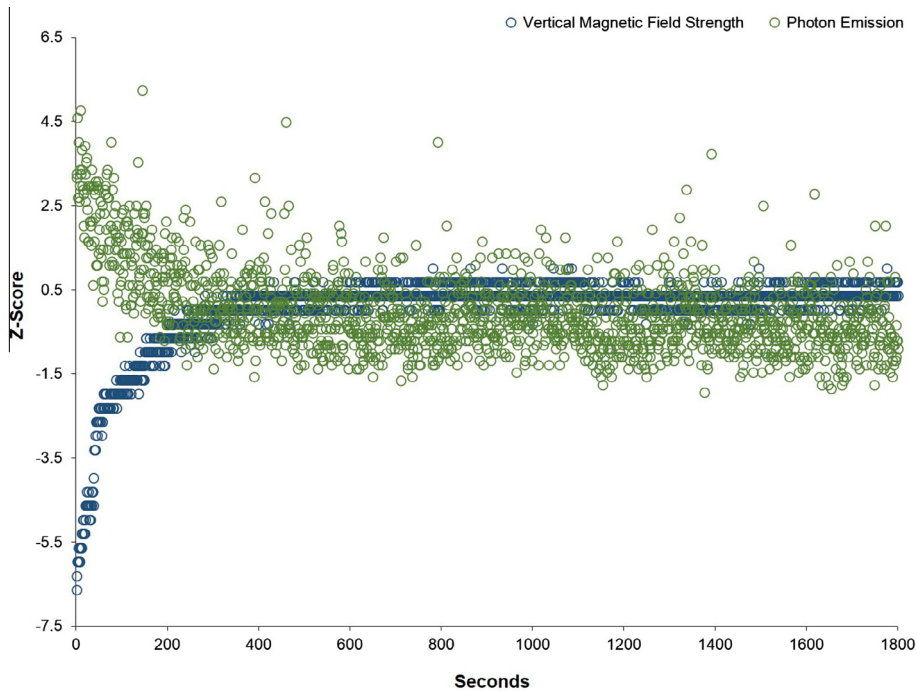
Fig. 7. Z-scores of distributions for a single experiment (run) over the 30 min interval (about 15–20 min after removal from incubator and 10 min after activation of measurements) for photon emissions (green) and the vertical magnetic field strength (blue) measured simultaneously near an aggregate of about 1 million melanoma cells.
