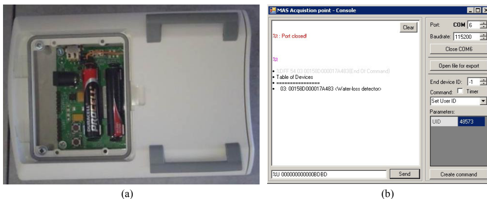
Fig. 3. (a) prototype of the wearable coordinator unit; (b) PC acquisition point software for controlling of sensor unit
