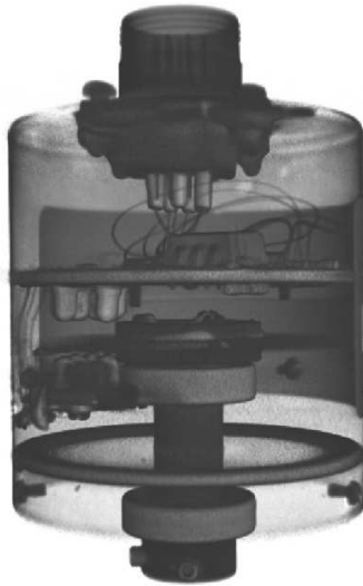
Fig. 9. CT scan of an optical encoder
