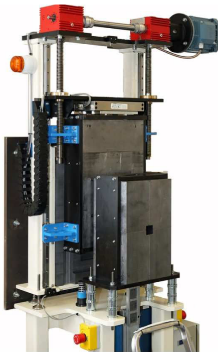
Fig. 4. Main shutter and automated aperture selector
