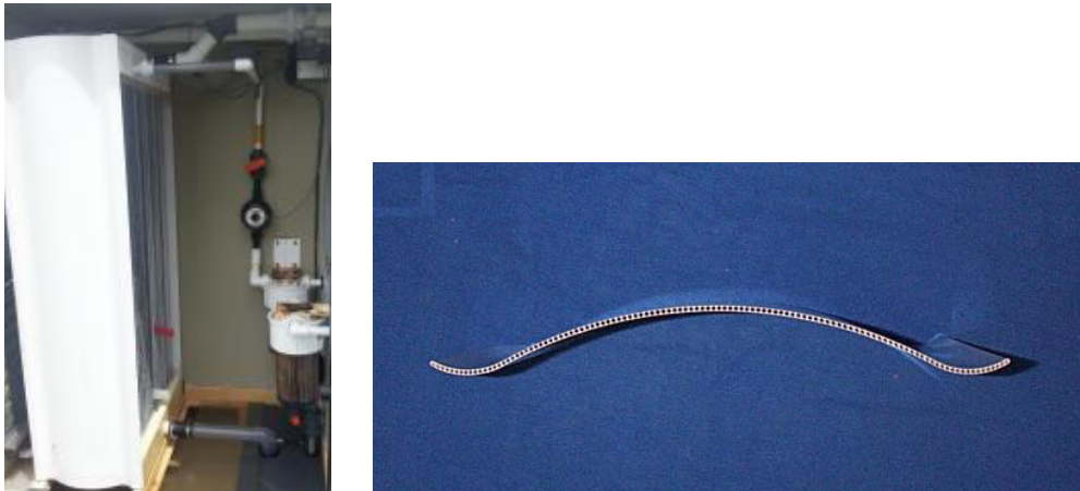
Fig. 2 (a) Internally cooled low-flow parallel plate falling-film conditioner; (b) top-view of a single plate showing the internal channels 6
