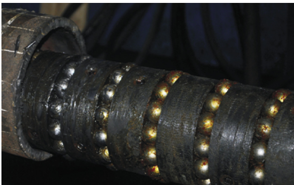
Fig. 2. Appearance of the spinning casing swage after repairing.
