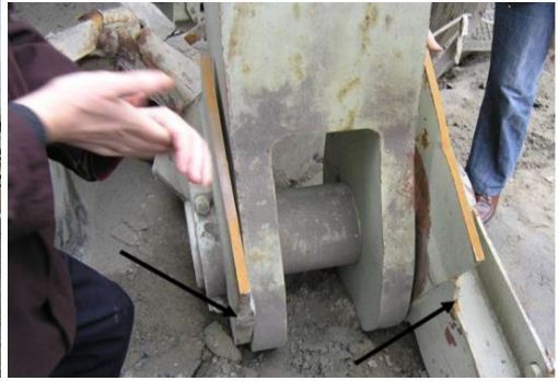
Fig. 2. Fracture of two lugs on counterweight holder
