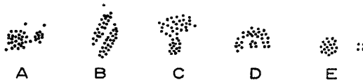
FIG. 1. Nagy (1968) has illustrated the major difficulties found in cluster analysis: (a) and (c) bridges between clusters; (b) nonspherical clusters; (d) linearly nonseparable clusters; (e) unequal cluster populations.
