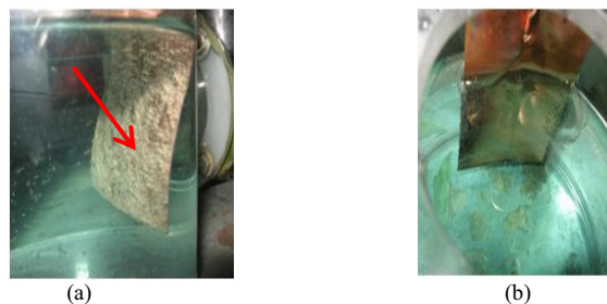
Fig. 4. Hydrogen bubbles formed on cathode on single chamber reactor (a) compared to clear solution on cathode compartment of partitioned reactor using water hyacinth leaf (b)
