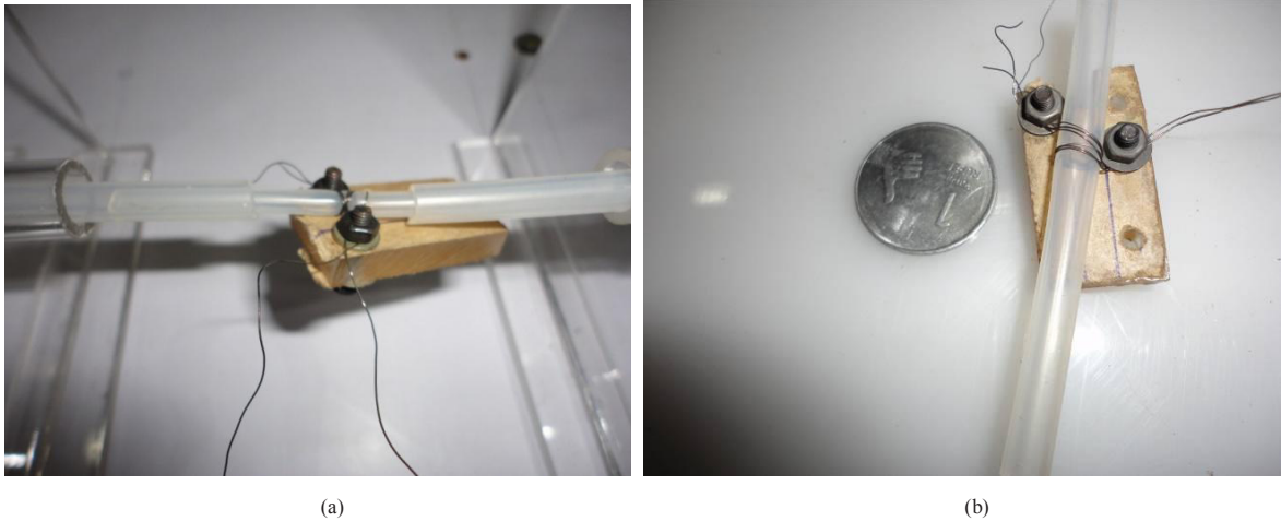
Figure 2 (a) Miniature Flexible SMA Wire Clamping; (b) Size representation of SMA Wire Clamp
