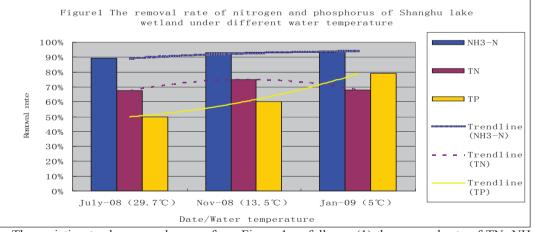
The variation tendency can be seen from Figure 1 as follows: (1) the removal rate of  $\overline{\text{TN}, \text{NH}_3-\text{N}}$ , and TP is different in the water body of Shanghu lake wetland, with the overall tendency of  $\text{NH}_3-\text{N} >$
