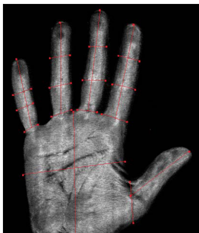
Fig. 3. The ultrasound image with some of the measurements taken in the classical Hand Geometry recognition method.
