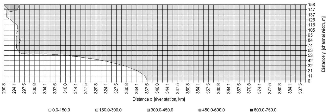
**Fig. 3.** Formation of the effluent plume with discharge site downstream from a preloaded tributary (Cl<sup>+</sup> mg L<sup>-1</sup>). (A) Near-shore discharge site and (B) mid-channel discharge site Elbe River below mouth of the Saale River. Approximate mixing calculation according to Fischer et al. (1979). Notice the differing scales of  $x$  and  $y$ .
