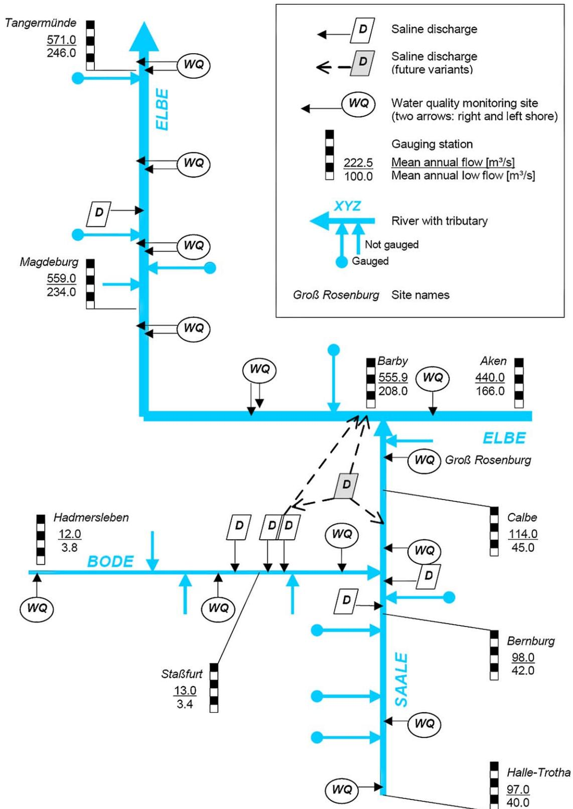
Fig. 1. Chloride model: conceptual schematic of the river system under study.
