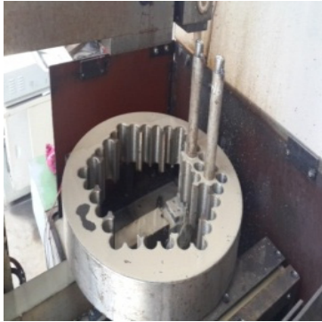
Fig. 3. EDM process of joints.
