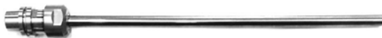
Figure 4. Tool holder and shank (L/D = 27, D = 10 mm, d = 8 mm) (not shown the cutter head at the right side)
