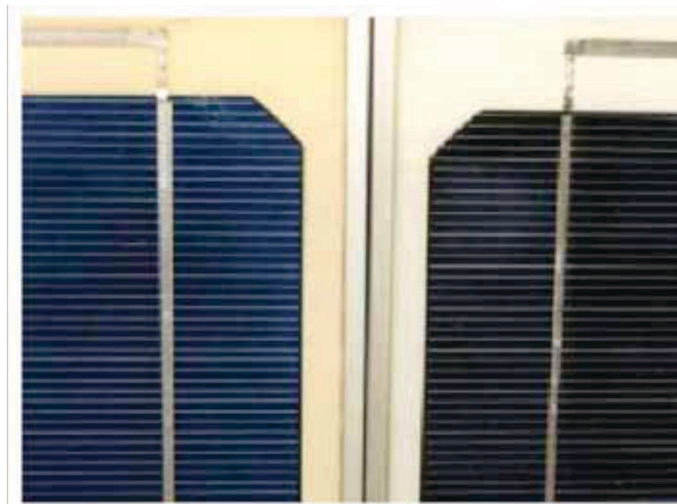
Fig. 2. Aged PV module after damp heat test (left) and unaged PV module as reference (right).
