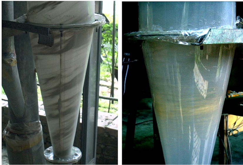
Fig. 18. Photos showing the trajectories of the tracing particles of different diameters (a) particles (raw material) flowing downward at the cone section and displaying a certain descending angle; (b) ceramic balls spinning at a certain height with almost zero descending angle.
