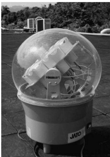
Fig. 9. Photo of solar concentrator employed in Wu et al. study. Reproduced from Ref. [121].
