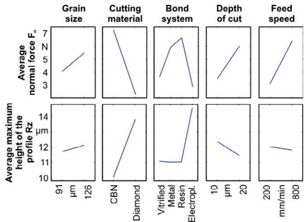
Fig. 9. Main effect plots for the grinded WC-Co coatings
