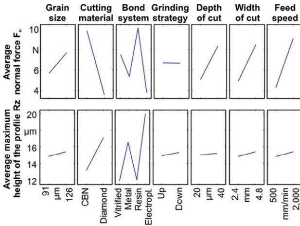
Fig. 6. Main effect plots for the grinded WC-Fe coatings
