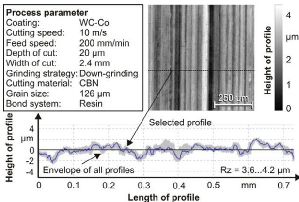
Fig. 7. Surface topography of a grinded WC-Co coating
