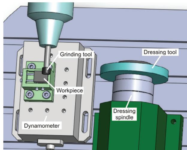
Fig. 3. Experimental setup
