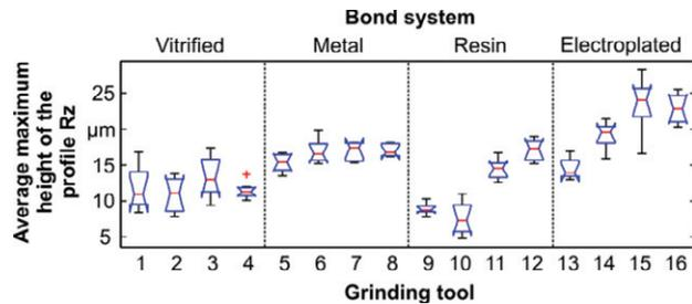
Fig. 5. Boxplot distribution of the roughness values Rz and the used grinding tools, as shown in Fig. 2, for the grinding of WC-Fe coatings
