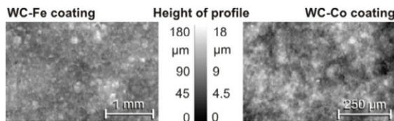
Fig. 1. Surface topographies of tungsten carbide coatings deposited by arc and HVOF spraying processes
