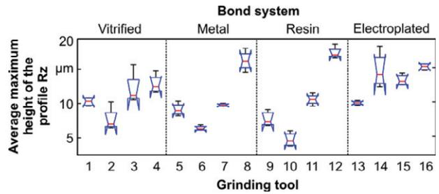
Fig. 8. Boxplot distribution of the roughness values  $R_z$  and the used grinding tools for the grinding of WC-Co coatings
