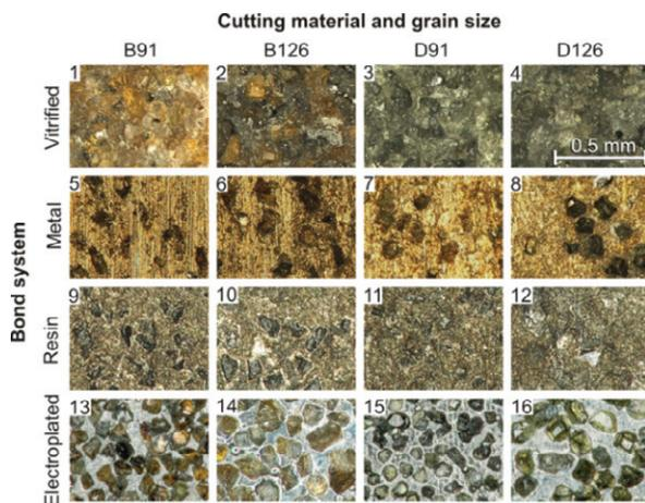
Fig. 2. Images of the applied grinding tools
