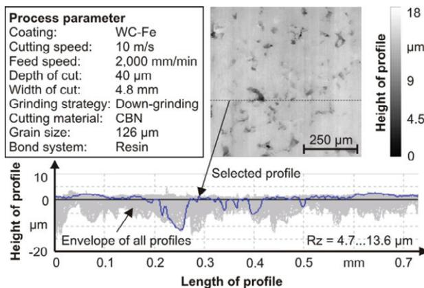
Fig. 4. Surface topography of a grinded WC-Fe coating
