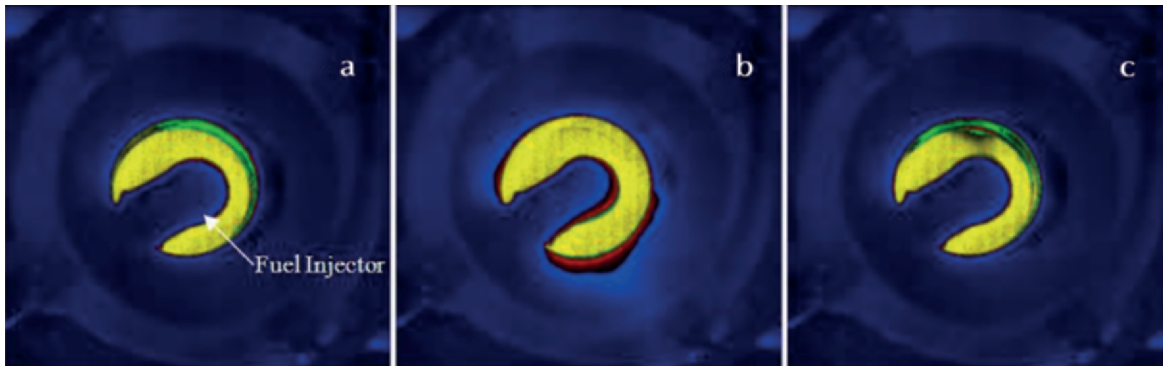
Figure 7. Case at 100 l/min gas, 100% premixed, a) the airflow is at 1,000 l/min. The flame is attached to the nozzle, b) the airflow is at 900 l/min. The flame is inside of the sleeve, close to flashback into the swirl chamber, c) the airflow is at 800 l/min. The flame is reattached to the nozzle again, out of the sleeve
