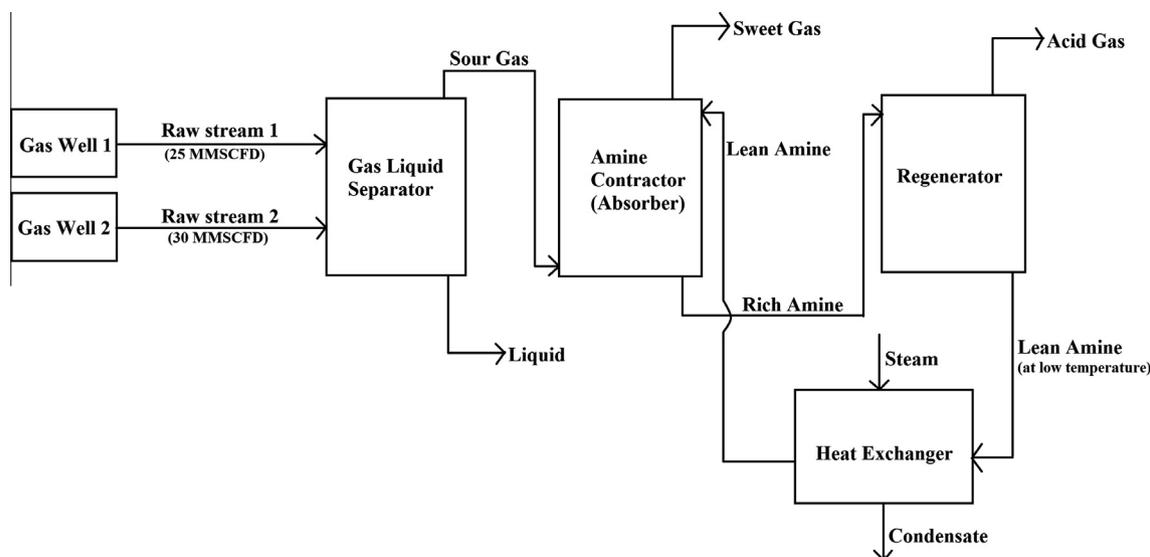
**Figure 1** Simplified flow-chart of gas sweetening unit.
