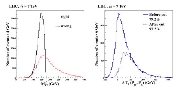
Figure 3. The distributions of  $T_2 \equiv M_{T2}^{t\bar{t}}$  (left panel) and  $\Delta T_2(P_W, P_R)$  (right panel), with  $P_W$  and  $P_R$  the wrong and right partitions respectively. The legend in the second panel indicates the percentage of correctly partitioned events, before and after inclusion of the cut  $M_T^{t\bar{t}}(0) > 400 \text{ GeV}$ , to be described in section 3.2.
