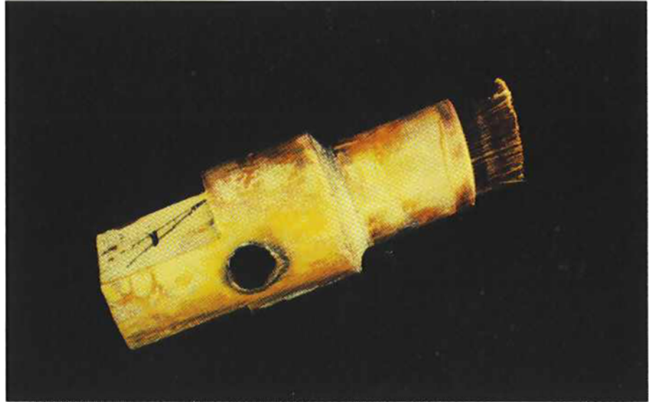
Fig. 1 A fibre brush made of gold fibres of about 0.5 cm length and 20 \mu\text{m} thickness, that is about one third that of a human hair, protruding from a copper matrix. The best data so far obtained, for example those incorporated in Figs. 6 to 8, were obtained with brushes of this type
