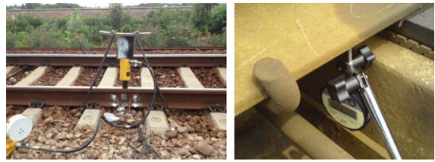
Fig. 2 Jack-loading diagram and vertical rail deflection measurement
